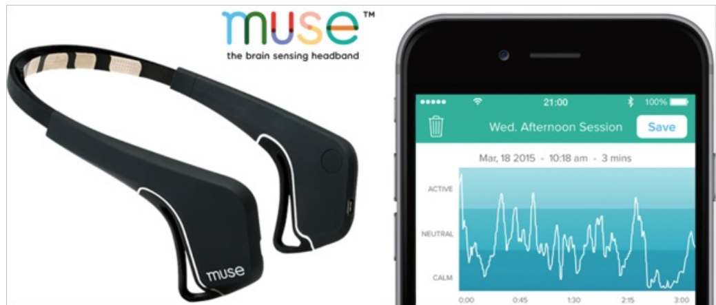
Figure 2: Novel applications of non-invasive brain electrodes. Muse, the brain brain sensing headband is an example of a commercial application of low resolution EEG to help improve meditation practices (Images by choose muse.com).
