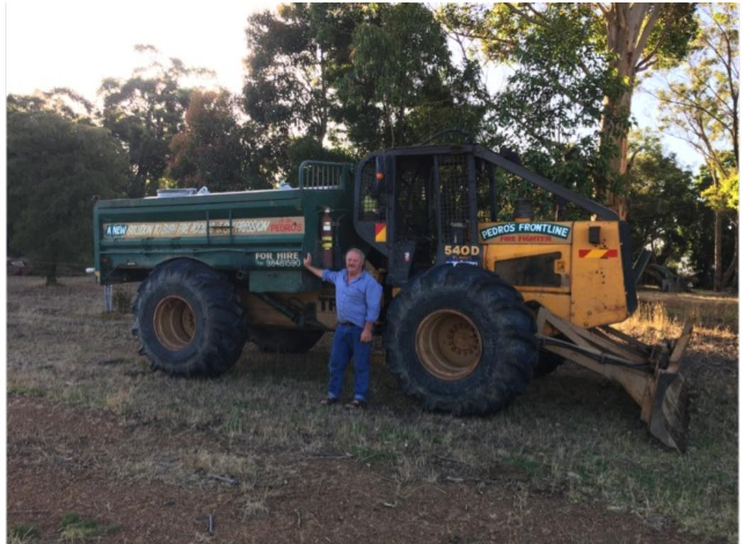
Figure 5: The author next to the fire-fighting unit built from a forestry log skidder: 'Pedro's Frontline Fire Fighter' (Photo: Anthony Kerr, 2017).
